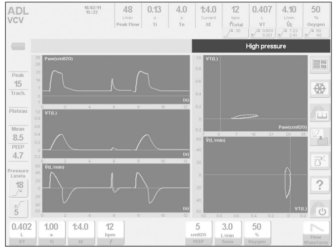
Fig. 4-6 Picture in which the space reserved for the emergence of On-screen notices of alarms is highlighted. In this case the alarm of Maximum inspiratory pressure is found to be active.
