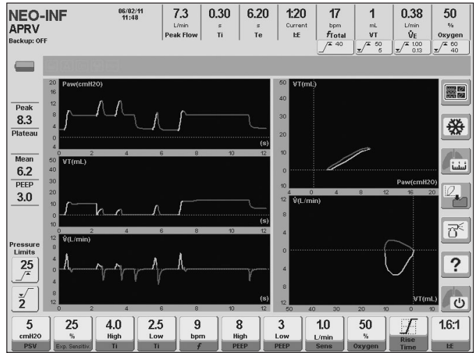
Fig. 10-17 APRV screenshot in NEO-INF. The picture shows that two spontaneous breaths have been carried out during the first high PEEP period, and another spontaneous respiration has been charted for the following low PEEP period.
