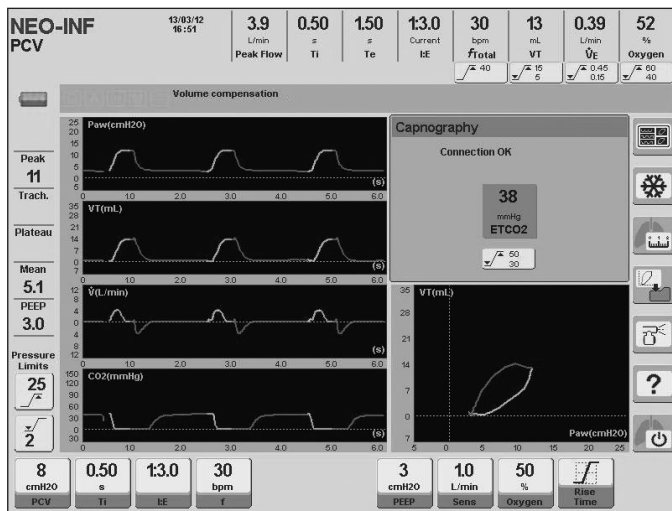
Fig. 14-3 Above: CAPNOGRAPHY screen for the ADL patient category. Incorporates two curves and one sheet of monitored data. Below: CAPNOGRAPHY screen for the NEO-INF patient category.
